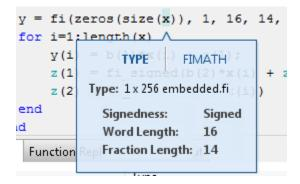
For a variable with a fixed-point type in the original code, when you place your cursor over the variable before or after conversion, the app displays the fixed-point type information.
